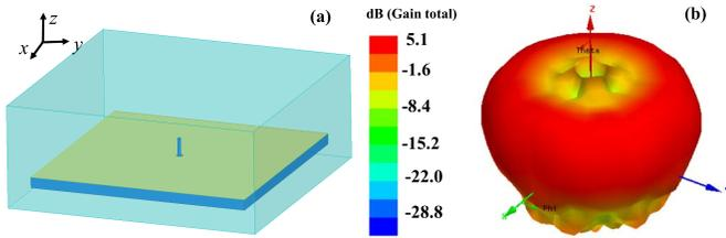
Fig. 2. (a) HFSS model of a quarter-wavelength monopole antenna on a finite ground ( $6 \times 6 \text{ mm}^2$ ) in the air box (radiation boundaries). The blue part is the  $290 \text{ } \mu\text{m}$  thick silicon substrate. (b) Radiation pattern of the monopole antenna at 160 GHz.
