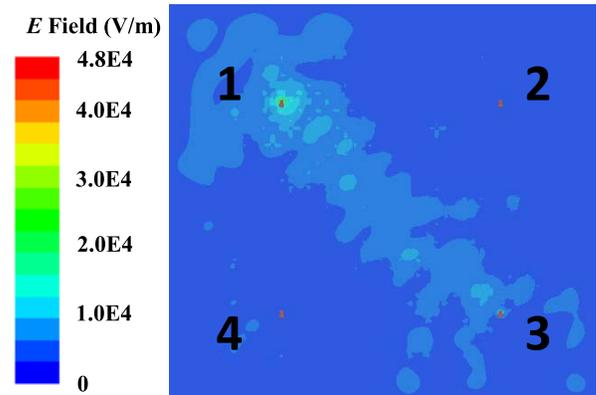
Fig. 9. Simulated  $E$  field (complex magnitude) distribution 0.5 mm above the ground plane when antenna 1 is excited at 60 GHz. The red dots are the locations of antennas. This figure shows that directional propagation is achieved between antenna 1 and antenna 3.
