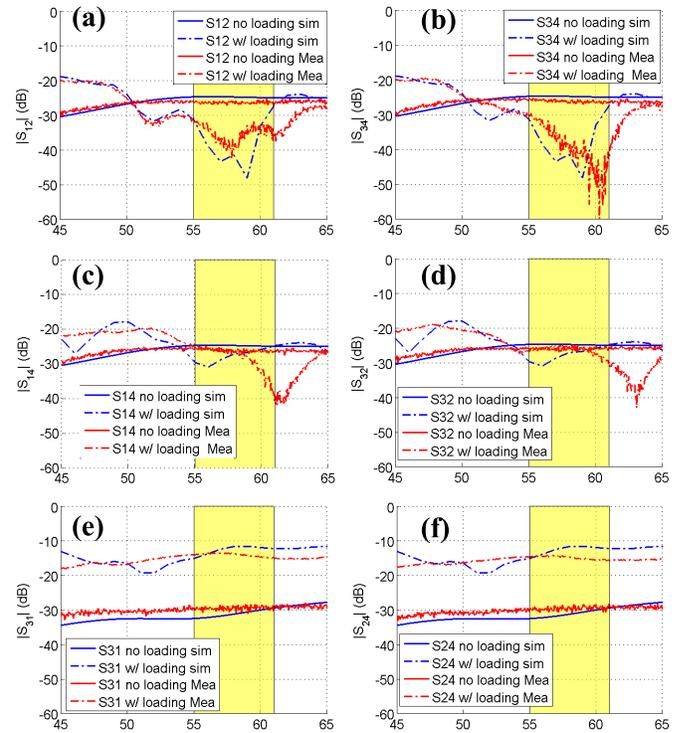
Fig. 16. Measured S-parameters of the fabricated monopoles in comparison with the simulation, with and without dielectric loading or metallic cover. (a)  $S_{12}$ , (b)  $S_{34}$ , (c)  $S_{14}$ , (d)  $S_{32}$ , (e)  $S_{31}$ , and (f)  $S_{24}$ .
