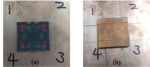
Fig. 13. (a) Four monopoles (indicated by the red squares) with the 3-D-printed polymer surrounding. (b) Final antenna structure with the metallic cover. The ground is  $152.4 \times 152.4$  mm<sup>2</sup> and 0.4 mm thick. The dielectric is  $18 \times 18 \times 1.25$  mm<sup>3</sup>. The four monopoles are at vertices of a  $12 \times 12$  mm<sup>2</sup> square. The top metallic cover has a dimension of  $20 \times 20 \times 0.4$  mm<sup>3</sup>.
