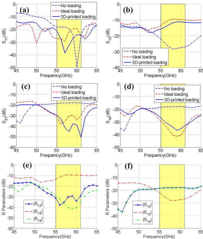
Fig. 7. S-parameters comparison of the no loading, the ideal dielectric blocks loading, and the 3-D-printed polymer loading cases. (a)  $S_{11}$ . (b)  $S_{13}$ . (c)  $S_{21}$ . (d)  $S_{14}$ . (e) S-parameters of the monopoles loaded with ideal dielectric blocks. (f) S-parameters of the no loading case.
