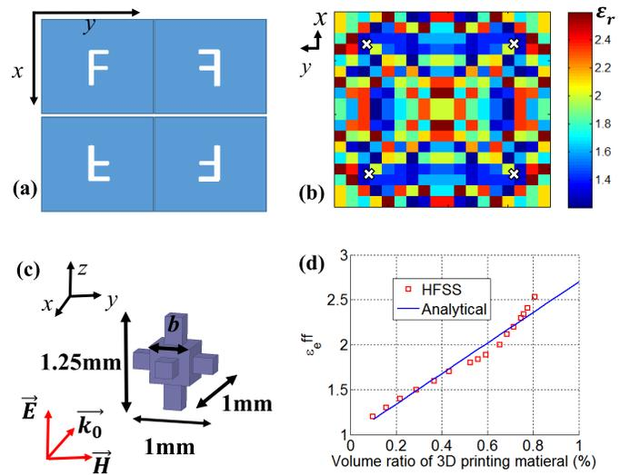
Fig. 5. (a) Symmetry used in the  $\epsilon_r$  distribution to reduce optimization parameters by a factor of four. The symmetry is with respect to the  $x$ - and  $y$ -axes. (b)  $\epsilon_r$  distribution surrounding the 60 GHz monopoles. The white crosses show the location of the monopoles. (c) Unit cell structure of the designed dielectric distribution. (d) Effective dielectric constant of unit cells with different polymer cube sizes based on the analytical calculation and HFSS simulation.
