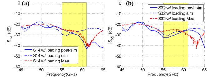
Fig. 17. Simulated S-parameters when the loaded dielectric is offset by  $(-0.3, 0.3, \text{ and } 0 \text{ mm})$  and the metallic cover is offset by  $(0.5, 0.5, \text{ and } 0 \text{ mm})$ . (a)  $S_{14}$  and (b)  $S_{32}$ .
