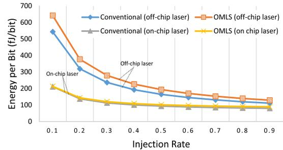
Fig. 3. Optimized energy consumption vs. injection rate of a link with 640 Gb/s bandwidth for different approaches.
